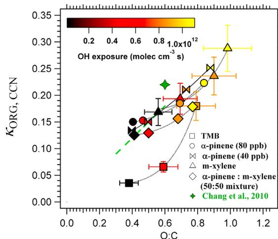
**Figure 2.**  $\kappa_{ORG,CCN}$  vs O:C for the laboratory SOA particles generated in this study. The  $\kappa_{ORG,CCN}$  for ambient OOA and the parameterization  $\kappa_{ORG,CCN} = (0.29 \pm 0.05) * O:C$  of Chang et al. [2010] (dashed line) are also plotted. Error bars (shown for m-xylene and TMB SOA only) represent measurement precision of  $\pm 15\%$  in  $\kappa_{ORG,CCN}$  and  $\pm 15\%$  in O:C.
