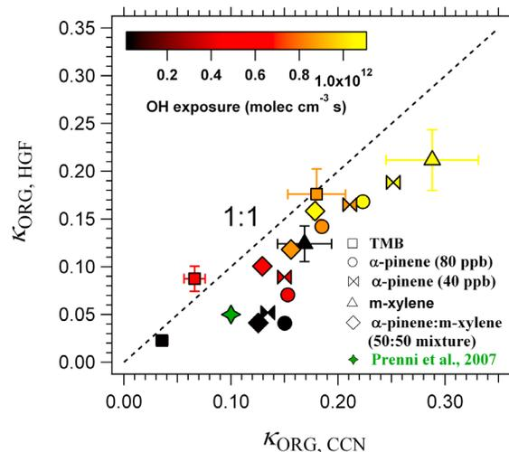
**Figure 3.**  $\kappa_{ORG,HGF}$  vs  $\kappa_{ORG,CCN}$  values for the laboratory SOA particles generated in this study. The error bars (shown for m-xylene and the TMB SOA only) represent measurement precision of  $\pm 15\%$  in  $\kappa_{ORG,CCN}$  and  $\pm 15\%$  in  $\kappa_{ORG,HGF}$ . Literature data from Prenni et al. [2007] is shown for comparison.
