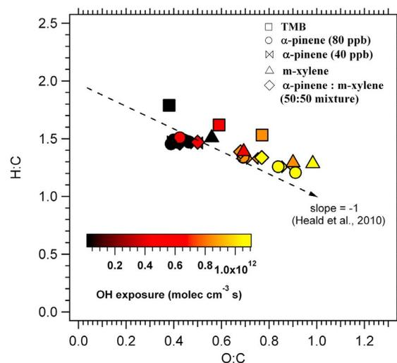
**Figure 4.** Elemental H:C vs O:C for the SOA systems plotted in Figures 1–3. For comparable OH exposure, the TMB particles have higher H:C than the other SOA types. The dashed line (H:C = 2, O:C = 1, from Heald et al. [2010]) is shown as a guide to the eye.
