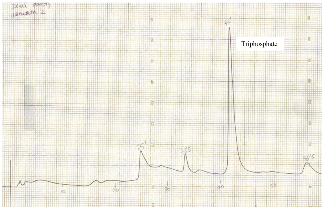
Figure 15. HPLC chromatogram of the crude mixture of dd2APyTP from an anion exchange column.
