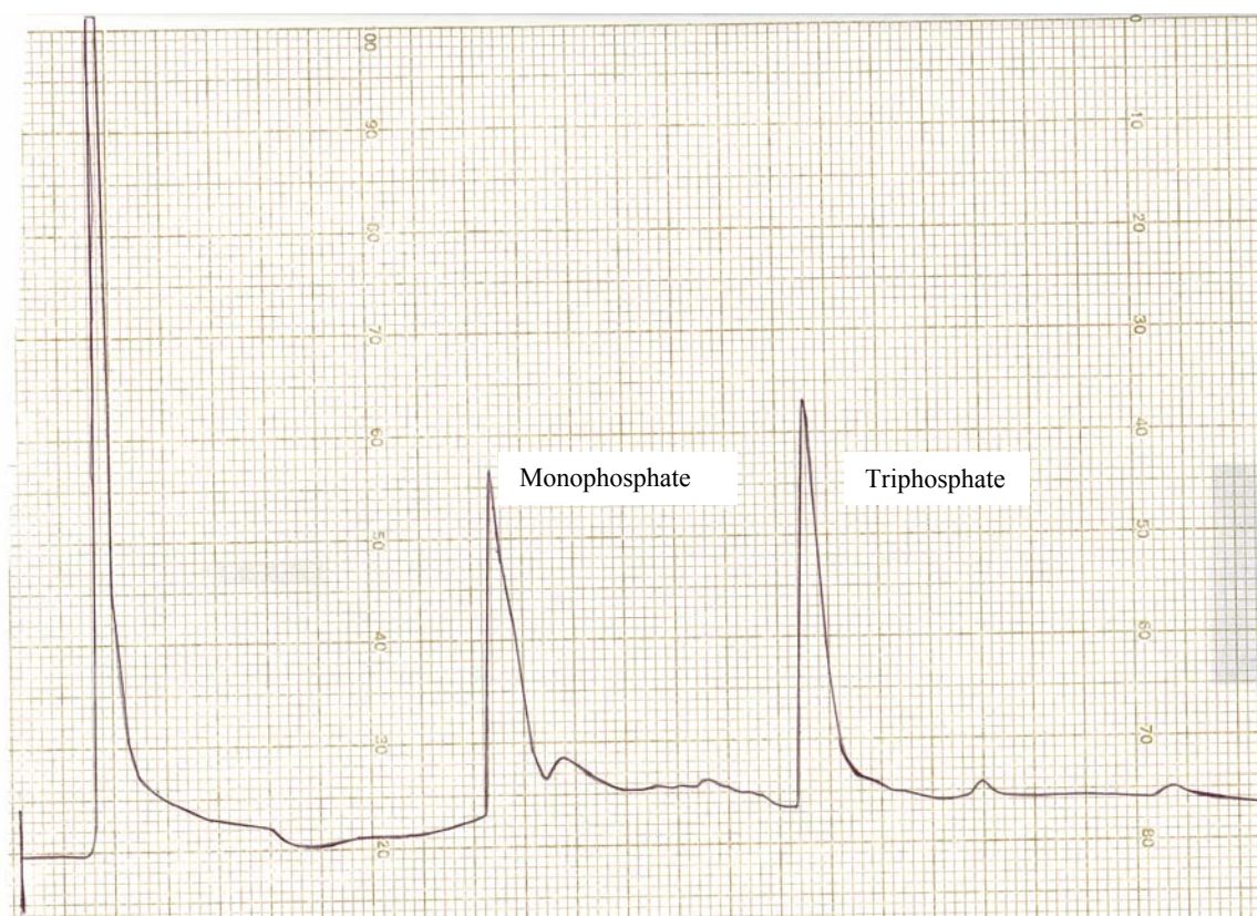
Figure 16. HPLC chromatogram of the crude mixture of 15 from an anion exchange column.
