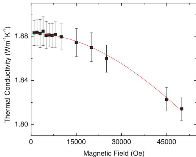
FIG. 4. (Color online) Thermal conductivity is plotted against magnetic field from 0.1 to 5 T and fit using Eq. (8) and  $\mu_d$  from Fig. 3. It is found that  $\kappa_{\text{lattice}} = 1.29 \text{ W mK}^{-1}$ .
