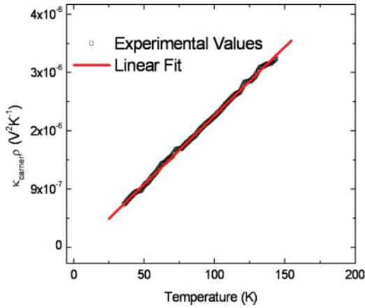
FIG. 6. (Color online)  $\kappa_{\text{carrier}}\rho$  is plotted against temperature from 35 to 150 K. The black points represent the measured data, while the red line is the linear fit. The slope of the linear fit provides the Lorenz number  $L = 2.21 \times 10^{-8} \text{ V}^2 \text{ K}^{-2}$ , and the y intercept gives  $\kappa_{\text{lattice}} = 2.14 \text{ W mK}^{-1}$ .
