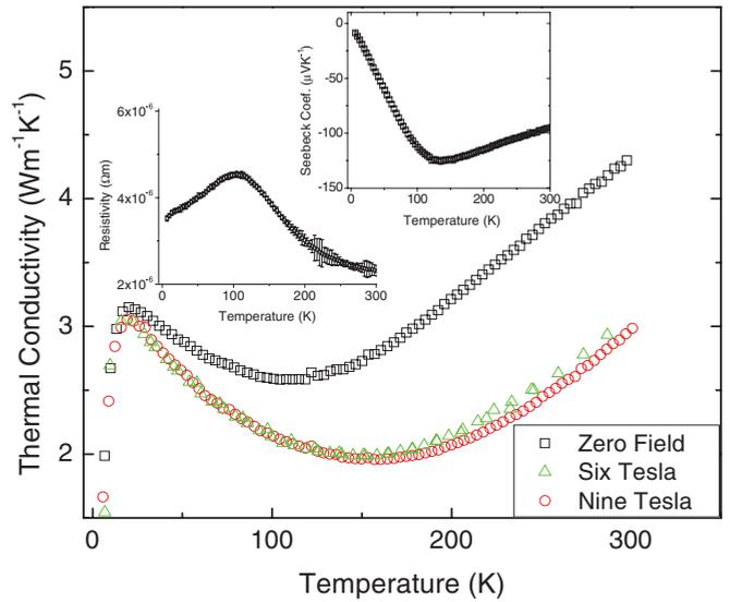
FIG. 5. (Color online) Thermal conductivity is plotted against temperature at magnetic fields of 0, 6, and 9 T for  $\text{Bi}_{0.88}\text{Sb}_{0.12}$ . The top right inset plots the Seebeck coefficient against temperature, while the top left inset plots  $r$  vs  $T$  from 5 to 300 K in zero magnetic field. It can be clearly seen that the bipolar contribution to the Seebeck coefficient becomes non-negligible around 150 K.
